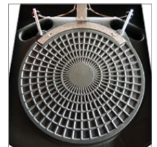
Recessed front bearing mounted turn plates.
